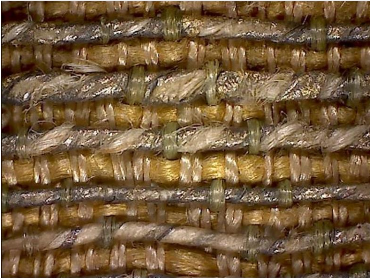
Image 2: Metal-coated membrane-based thread wefts (magnified view). Textile fragment, Italy, 14 th c.; Cooper Hewitt, Smithsonian Design Museum, 1902-1-329a. Image by Cristina Scibè, Museum Conservation Institute, Smithsonian Institution.
