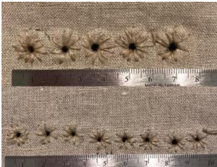
Photo 2: Materials testing. Top row: 9mm internal diameter metal rings stitched with 2/10 linen. Bottom row: 5mm internal diameter metal rings stitched with 2/10 linen. Both sample rows are stitched in a frame, sandwiched between 4 layers of 200 gsm linen. Photo by Jack Paltanen. Copyright Blue Trillium Textiles, 2021.
